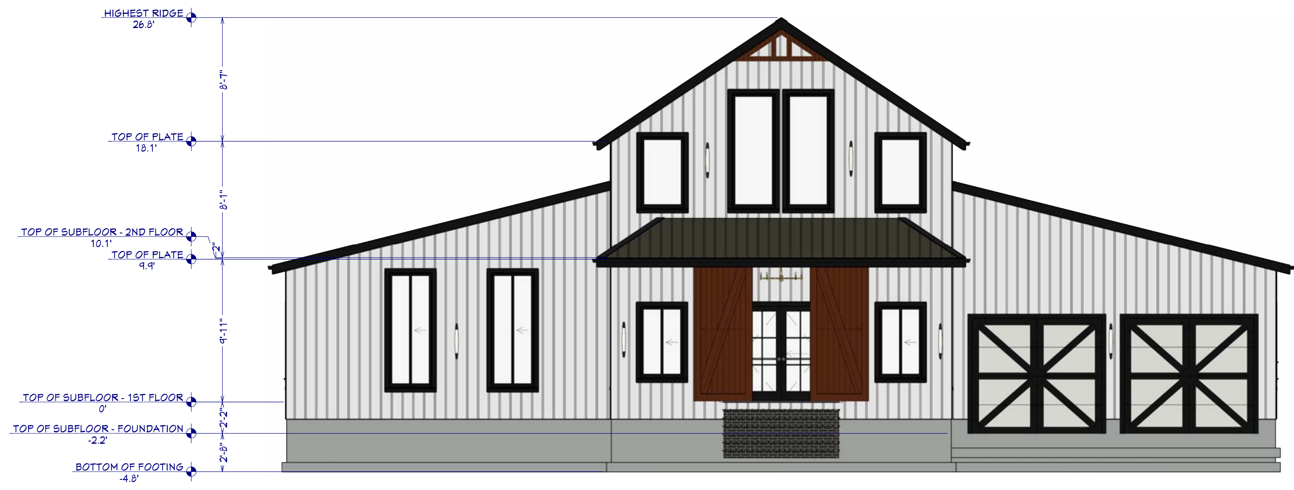
Exterior Elevation Front
